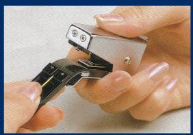
Bending the leaf spring to break the fibre end.
